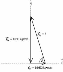
From the figure above, careful measurements give  $p_{C_f} = 0.22$  kg·m/s and  $\theta = 72.5^{\circ}$  N of W.
