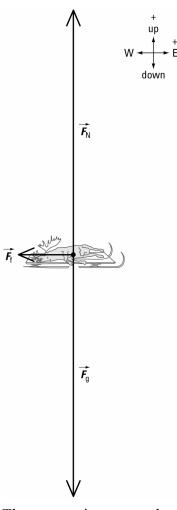
The system is not accelerating up or down. So in the vertical direction,  $F_{\text{net}_v} = 0 \text{ N}$ .
