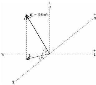
Use the tangent function to find the direction of  $\vec{v}_{C_f}$  in the east-north plane.
