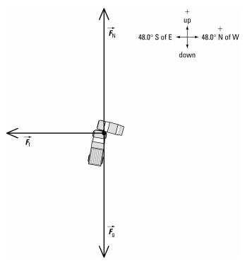
The system is not accelerating up or down. So in the vertical direction,  $F_{\text{net}_v} = 0 \text{ N}$ .
