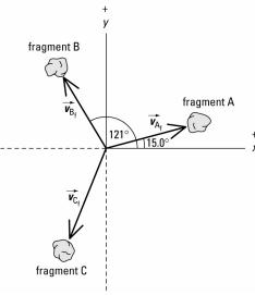
Fragment C will move  $15^{\circ} + 53^{\circ} + 180^{\circ} = 248^{\circ}$ .
