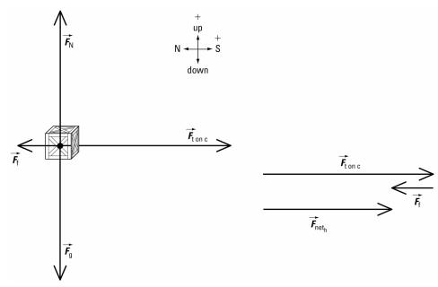
The crate is not accelerating up or down. So in the vertical direction,  $F_{\text{net}_{v}} = 0 \text{ N}$ .
