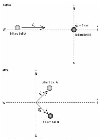
At the instant the billiard balls collide, only one point on the surface of ball A is in contact with ball B. If you were to draw a tangent through this point of contact, you would find that the impulsive forces act perpendicular to the tangent and these forces act along the line joining the centres of both balls.
