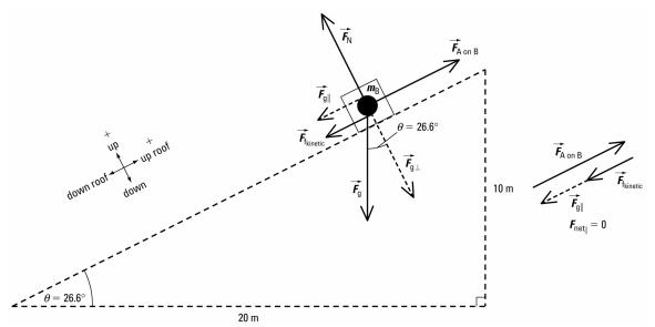
Since bundle B is moving at constant speed up the roof,  $\vec{F}_{net} = 0$  N both parallel and perpendicular to the roof.
