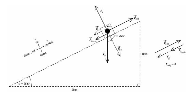
Since the system is moving at constant speed up the roof,  $\vec{F}_{net} = 0$  N both parallel and perpendicular to the roof.
