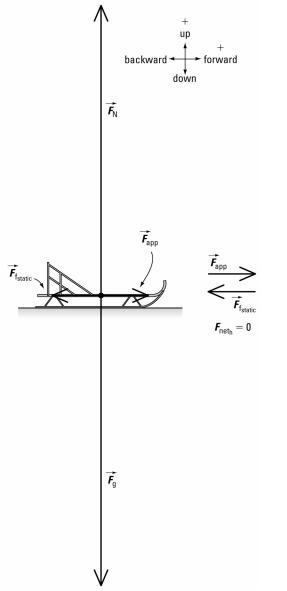
Since the sled is not accelerating in the vertical direction,  $F_{\text{net}_h} = 0$  N. Write equations to find the net force on the sled in both directions. horizontal direction vertical direction
