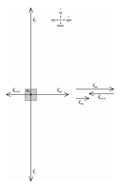
Box A is not accelerating up or down. So in the vertical direction,  $F_{\text{net}_v} = 0$  N.
