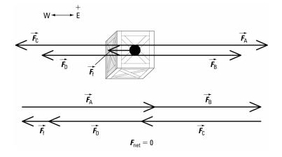
To determine the direction of  $\vec{F}_{f}$ , first determine  $\vec{F}_{net}$  if there were no friction.  $\vec{F}_{net_{no fric}} = \vec{F}_{A} + \vec{F}_{B} + \vec{F}_{C} + \vec{F}_{D}$
