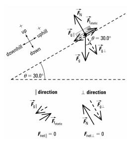
Since the system is not accelerating,  $\vec{F}_{net} = 0$  N both parallel and perpendicular to the incline.
