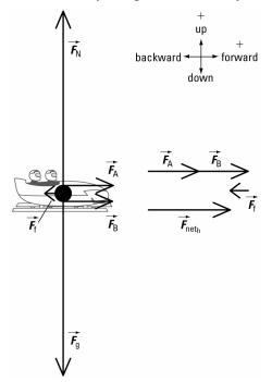
The system is not accelerating up or down. So in the vertical direction,  $F_{\text{net}_v} = 0$  N.
