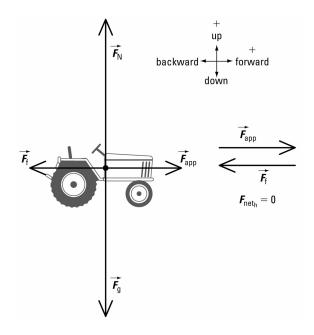
Since the tractor is not accelerating in the vertical direction,  $F_{\text{net}_h} = 0$  N. Write equations to find the net force on the tractor in both directions. horizontal direction vertical direction
