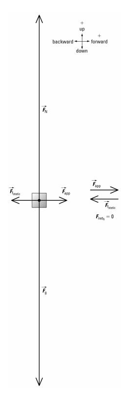
Since the block is not accelerating,  $\vec{F}_{net} = 0$  N in both the horizontal and vertical directions.
