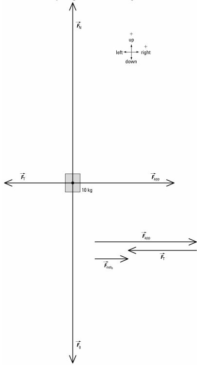
The block is not accelerating up or down. So in the vertical direction,  $F_{\text{net}_v} = 0$  N.
