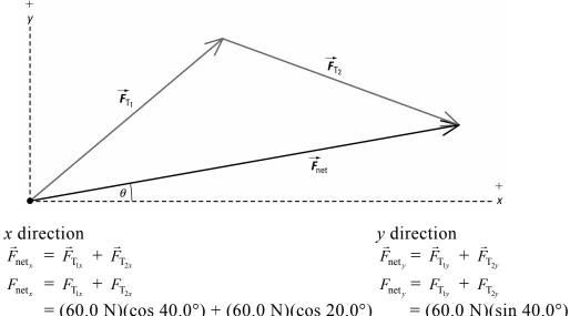
$$= (60.0 \text{ N})(\cos 40.0^{\circ}) + (60.0 \text{ N})(\cos 20.0^{\circ}) = (60.0 \text{ N})(\sin 40.0^{\circ}) + \{-(60.0 \text{ N})(\sin 20.0^{\circ})\} = 102.3 \text{ N} = 18.05 \text{ N}$$
