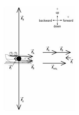
The system is not accelerating up or down. So in the vertical direction,  $F_{\text{net}_v} = 0$  N. Write equations to find the net force on the system in both the horizontal and vertical directions.
