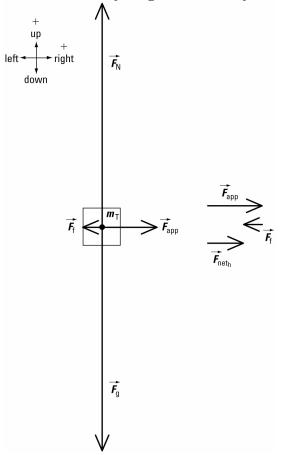
The system is not accelerating up or down. So in the vertical direction,  $F_{\text{net.}} = 0$  N.
