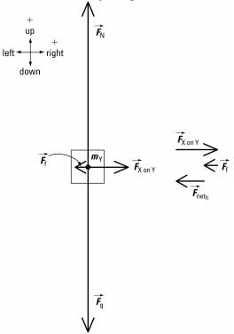
Block Y is not accelerating up or down. So in the vertical direction,  $F_{\text{net}_v} = 0$  N.
