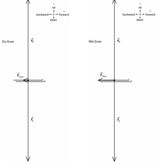
Since the skis are not accelerating,  $\vec{F}_{net} = 0$  N both in the horizontal and vertical directions.
