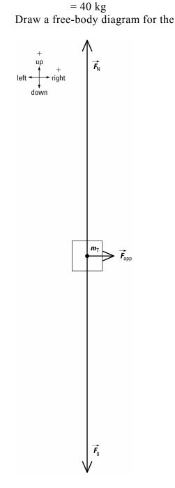
The system is not accelerating up or down. So in the vertical direction,  $F_{\text{net}_v} = 0$  N.
