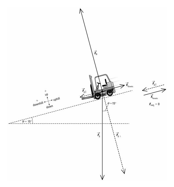
Since the lift truck is moving at constant speed downhill,  $\vec{F}_{net} = 0$  N both parallel and perpendicular to the incline.
