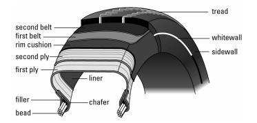
Traction is the force of friction, exerted by the tire tread on a road surface, that provides grip. Traction is determined by measuring the force needed to start dragging a tire over a road surface. This force depends on the temperature of the road surface and the tire, and the nature of the road surface, e.g., dry concrete, dry asphalt, packed snow, black ice, or a surface covered with a layer of water. Coefficients of static and kinetic friction are measured for different tire tread
