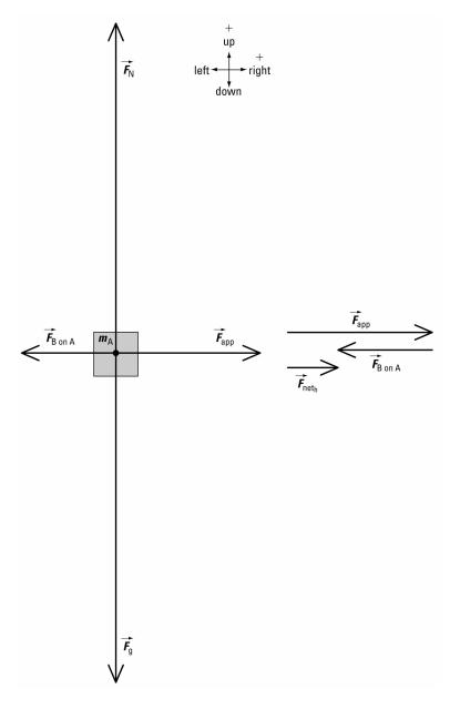
Log A is not accelerating up or down. So in the vertical direction,  $F_{net_v} = 0$  N.
