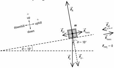
Since the crate is not accelerating,  $\vec{F}_{net} = 0$  N both parallel and perpendicular to the incline.
