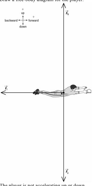
The player is not accelerating up or down. So in the vertical direction,  $F_{\text{net}_v} = 0$  N.
