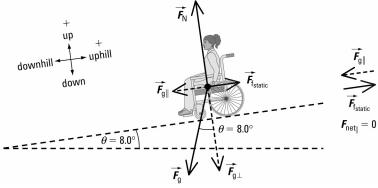
Since the wheelchair is not accelerating,  $\vec{F}_{net} = 0$  N both parallel and perpendicular to the incline.
