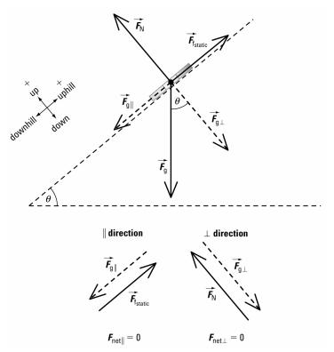
Since the loonie is not accelerating,  $\vec{F}_{net} = 0$  N both parallel and perpendicular to the incline.
