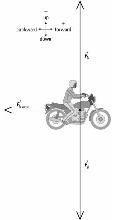
Since the system is skidding,  $\vec{F}_{net} \neq 0$  N in the horizontal direction, but  $\vec{F}_{net} = 0$  N in the vertical direction.
