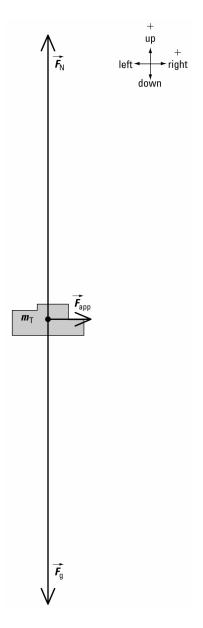
The system is not accelerating up or down. So in the vertical direction,  $F_{\text{net}_v} = 0$  N.
