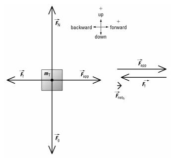
The system is not accelerating up or down. So in the vertical direction,  $F_{\text{net}_v} = 0$  N.
