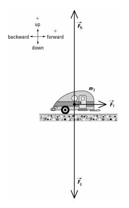
The trailer is not accelerating up or down. So in the vertical direction,  $F_{\text{net}_v} = 0$  N.
