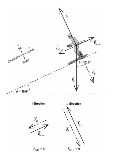
When the angle of the incline is just enough for the skier to start moving, the surface of the incline is exerting the maximum magnitude of the force of static friction on the skier.
