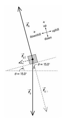
Since the block is accelerating downhill,  $\vec{F}_{net} \neq 0$  N parallel to the incline, but  $\vec{F}_{net} = 0$  N perpendicular to the incline.
