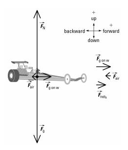
The car is not accelerating up or down. So in the vertical direction,  $F_{\text{net}_v} = 0$  N.
