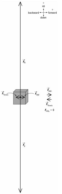
Since the crate is moving at constant speed,  $\vec{F}_{net} = 0$  N in both the horizontal and vertical directions.
