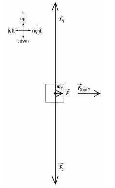
Block Y is not accelerating up or down. So in the vertical direction,  $F_{\text{net}_v} = 0$  N.
