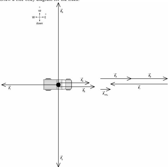
The truck is not accelerating up or down. So in the vertical direction,  $F_{\text{net}_v} = 0$  N.
