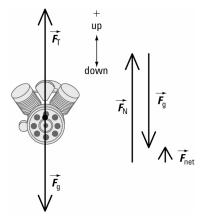
The engine is not accelerating left or right.
