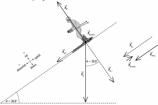
Since the skier is accelerating downhill,  $\vec{F}_{net} \neq 0$  N parallel to the incline, but  $\vec{F}_{net} = 0$  N perpendicular to the incline.
