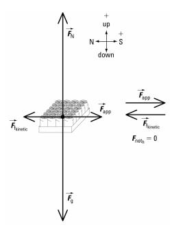
Since the case is moving at constant speed,  $\vec{F}_{net} = 0$  N in both the horizontal and vertical directions.
