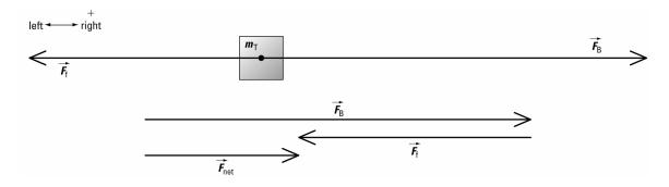
$\vec{F}_{\rm B}$  is equal to the gravitational force acting on  $m_{\rm B}$ .
