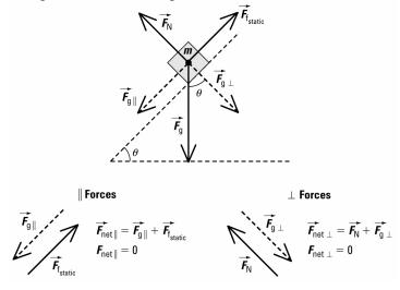
Students must explain why they used the sine and cosine of the angle to determine the parallel and perpendicular components respectively.
