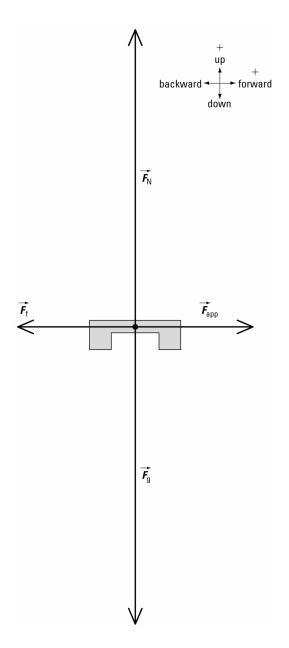
Since the slider is not accelerating,  $\vec{F}_{net} = 0$  N in both the horizontal and vertical directions.
