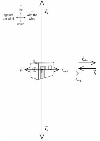
The hut is not accelerating up or down. So in the vertical direction,  $F_{\text{net}_{u}} = 0$  N.
