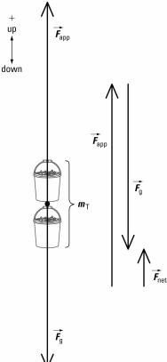
The system is not accelerating left or right. So in the horizontal direction,  $F_{net_n} = 0$  N. For the vertical direction, write an equation to find the net force on the system.
