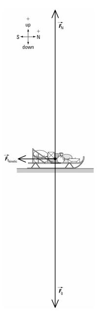
Since the sled is coasting,  $\vec{F}_{net} \neq 0$  N in the horizontal direction, but  $\vec{F}_{net} = 0$  N in the vertical direction.
