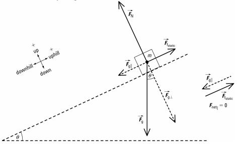
Since the box is not accelerating,  $\vec{F}_{net} = 0$  N both parallel and perpendicular to the incline.
