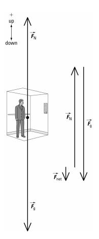
The system is not accelerating left or right. So in the horizontal direction,  $F_{\text{net}_h} = 0$  N.
